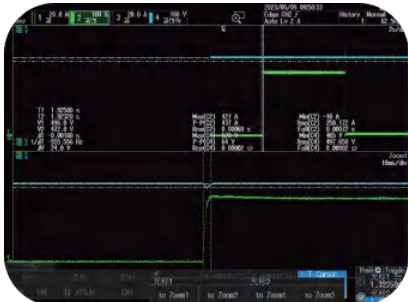
Sudden loading at 500V, voltage fluctuation: 24V@400A
